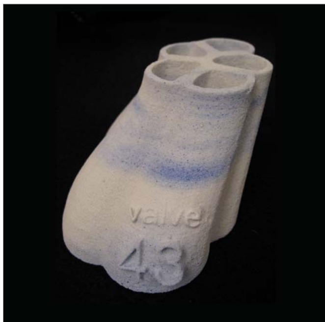
“Valve 43” is a sculpture created by Meghan Trainor, a graduate student in the UW’s Center for Digital Arts and Experimental Media. She designed the piece in Rhino 3D and was the first to use the new Vitraglyphic process to produce objects other than test shapes.
